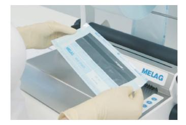
The **weekly** seal check verifies the quality of the seal seam in accordance with DIN EN ISO 11607-2.
