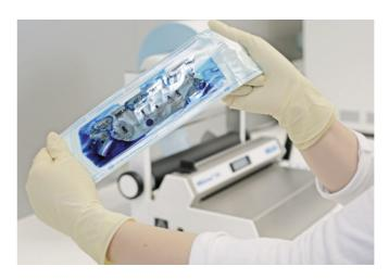
The MELA*ink* test is a reliable test for performing a weekly routine check of the seal seam for leaks in accordance with DIN EN ISO 11607-1 and ASTM F1929-12.
