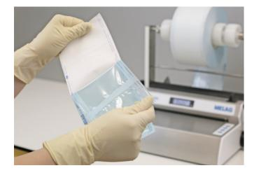
Please make sure to carry out the peel test on a **daily** basis, preferably before starting work: The tested seal seam must be even and complete.
